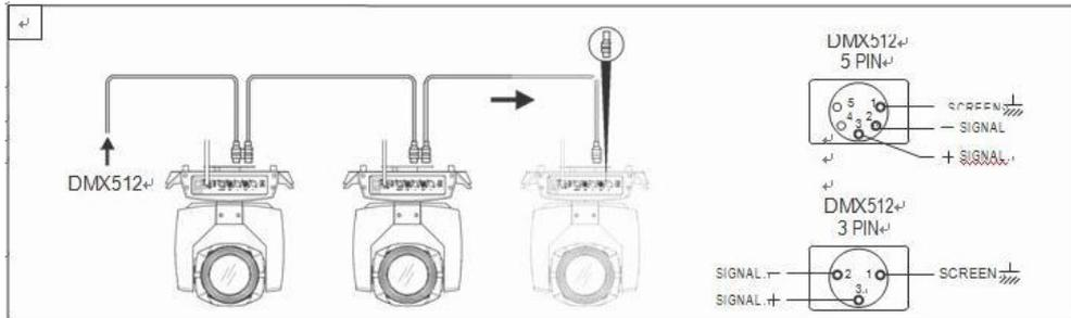
picture1 DMX signal line connection diagram
