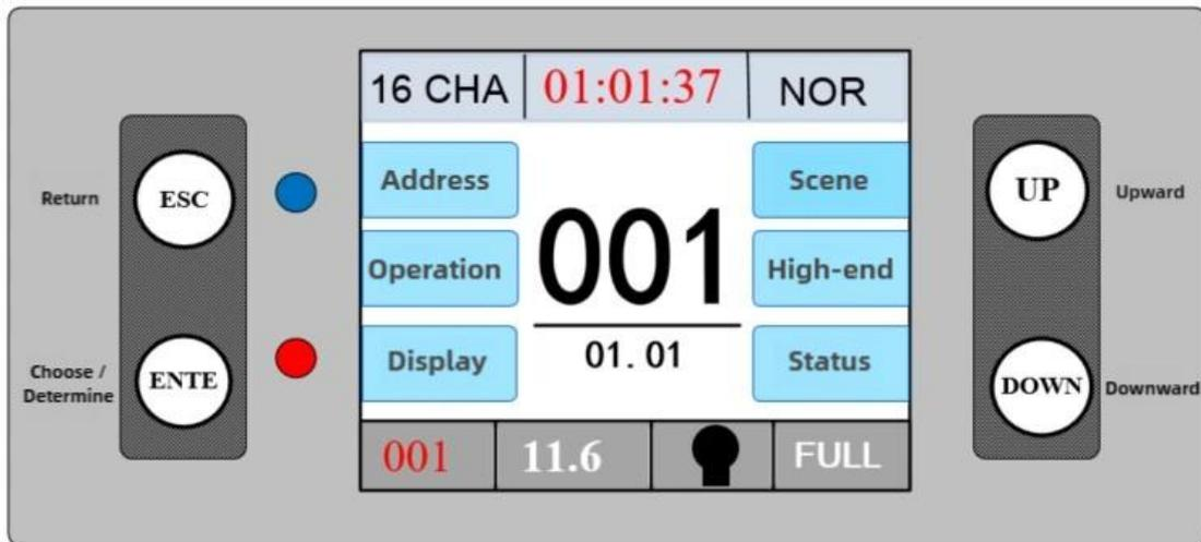
picture3-1 Schematic diagram of touch button display panel
